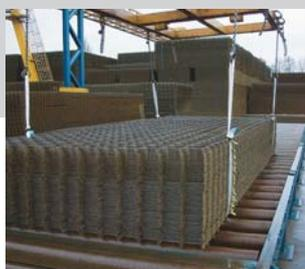
The product stored with the sling. It is **not necessary to resling**.
