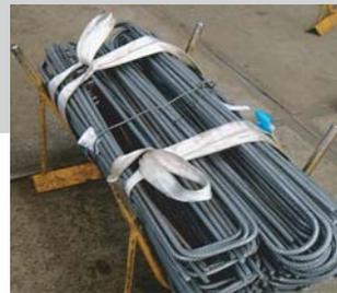
The **sling** is only **placed once** in the transport process. The **product** is **carried** throughout the factory with the **same sling**.
